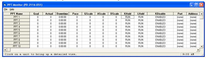
We need to tell the PPT monitor software about the network of PPTs connected to the PC. Click on the **[File]** menu and then select **[Configure PPTs...]**.
