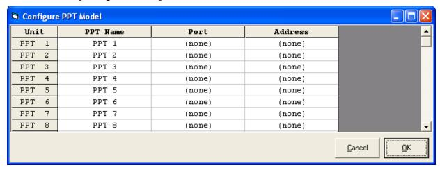
The Configure PPTs screen is where you tell the monitoring software about all of the AF-27xx-xxx PPTs connected to the PC, and how to communicate with them. The PPT monitoring software can manage up to sixty four PPTs.
