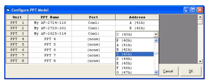
In the above example, the monitoring software is directed to gather data from three PPTs (My AF-2724-116, My AF-2720-101, and My AF-2625-314). All three PPTs are connect to the PC's COM1: serial port. My AF-2724-116 PPT has an assigned address of A 41h. My AF-2720-101 has an assigned address of B 42h. The AF-2625-314 has an assigned address of C 43h.
