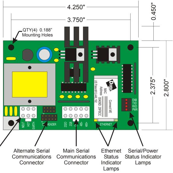
The ESB is constructed by integrating a Digi Connect ME Ethernet module with a 120VAC linear power supply and RS-232/485 serial communications transceiver.
